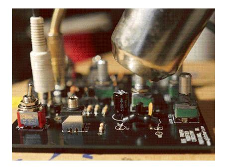
First, place the photocell, solder it and bend it down to the PCB.
