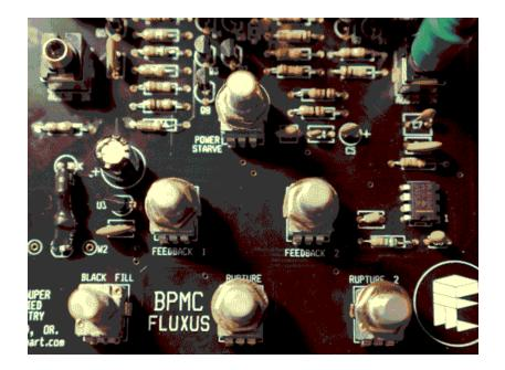
Second, let's place all the capacitors that are not polarity sensitive. Place, solder and trim leads. Ignore the polarity marker next to C5. It does not matter.
